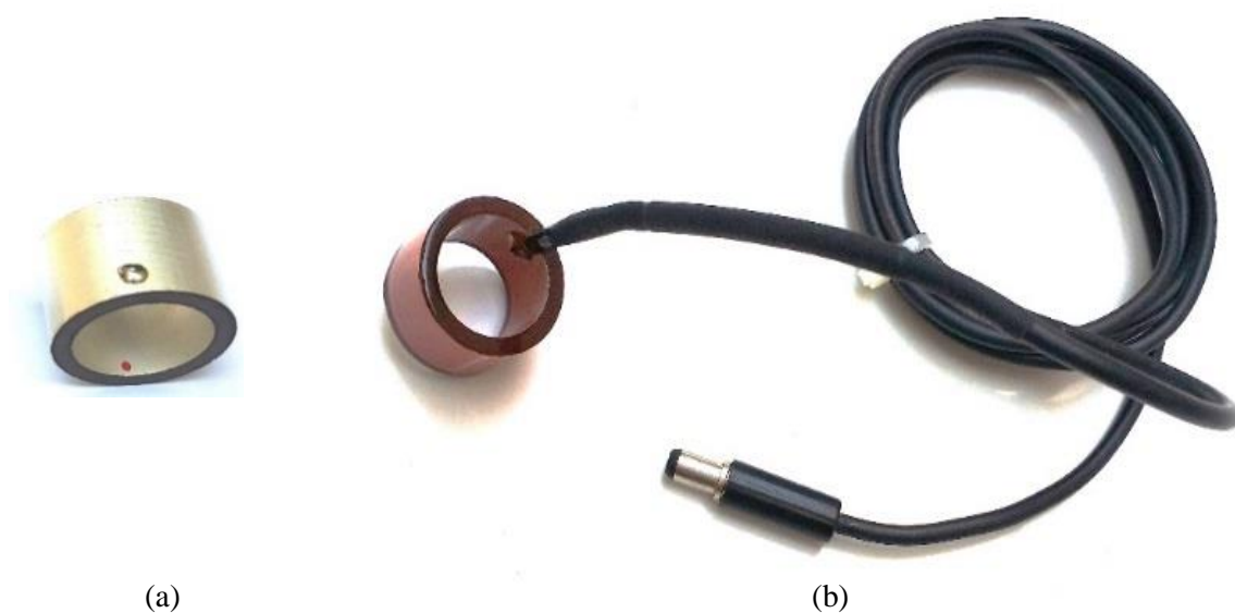
Figure 3.2. (a) Raw piezo-ceramic element (b) Water-proof underwater acoustic transducer.
