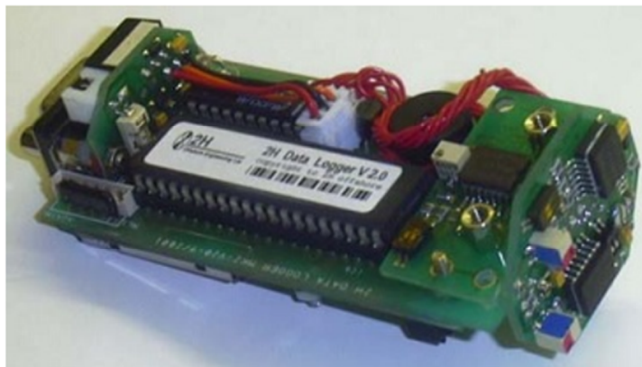
Figure 1-2. 2H Data Logger [5]. A standalone data logger is a data-capturing device that can automatically log data and store it in its on-board memory for a later processing of data stored in memory (e.g. a computer).
