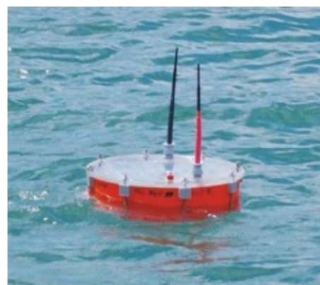
Figure 1-8. Gateway [21]. Gateway is same as the sensor node with additional long-range RF communication capability to communicate with the base station.
