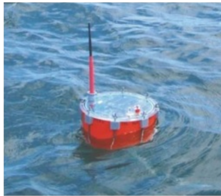
Figure 1-7. Sensor Node [21]. It is composed of control unit and data processing, signal acquisition and conditioning, local transmission radio, energy-harvesting mechanisms, and energy storage
