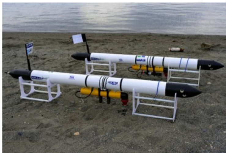
Figure 1-4. eFolaga AUVs Equipped with KM Modems [15]. These are surveillance AUVs controlled from a remote station to respond against any intrusion.
